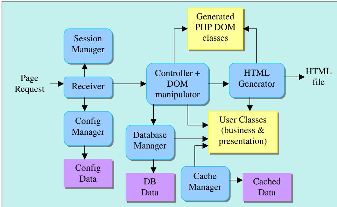
Fig 2 Data Flow Diagram for Request Processing
