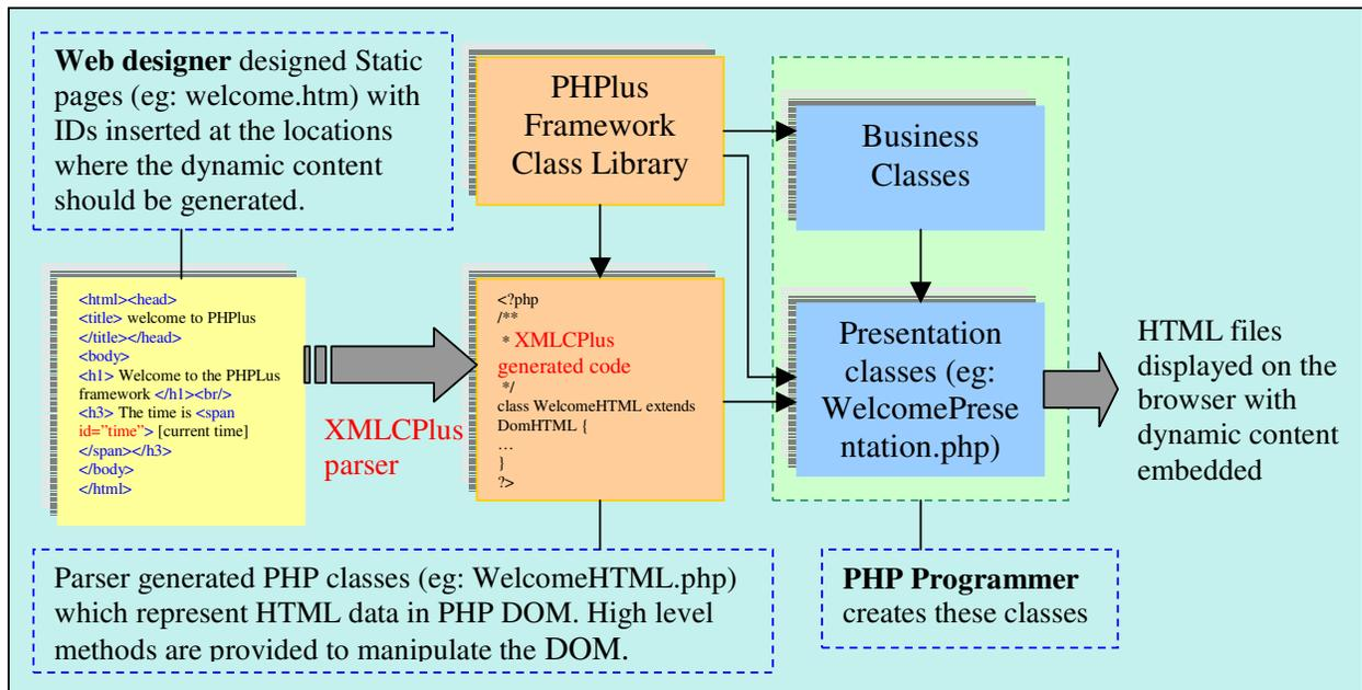
Fig 2 Work Flow Involved in Using the PHPlus Framework
